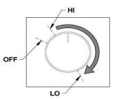
When using the optional blower, allow the stove to reach operating temperature (approximately one hour), before turning it on. The increased airflow from the blower cools the firebox and could affect the start-up combustion efficiency if the blower is turned on too early.
