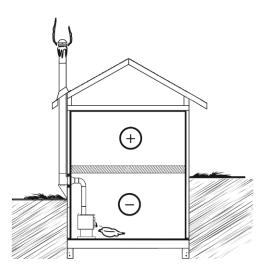
Good System Design Inside chimneys are preferred because even when no fire is burning, there is normally upward flow in the system.
