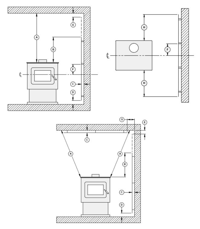
**Clearances for shield construction**
