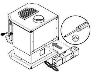
Your blower has a rheostat, see the illustration on the right to identify the different adjustment positions; either from high (HI) to low (LO) or closed (OFF).
